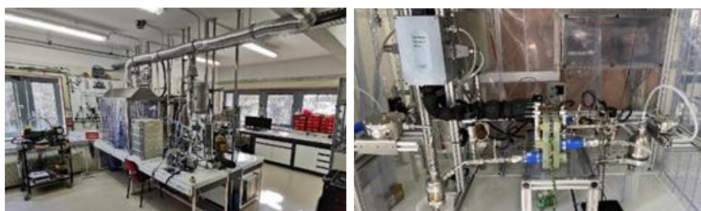
Short-stack test bench of Centre PERSEE/Mines Paris PSL.
